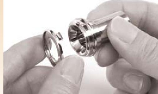
Place retained Gasket over gland face. Be careful not to scratch or nick sealing surface as this could affect performance.
