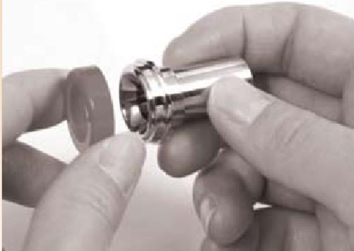
Remove plastic protector cap protecting the gland sealing surfaces. Go to STEP2A for Retainer Assembly, other go to STEP2B.
