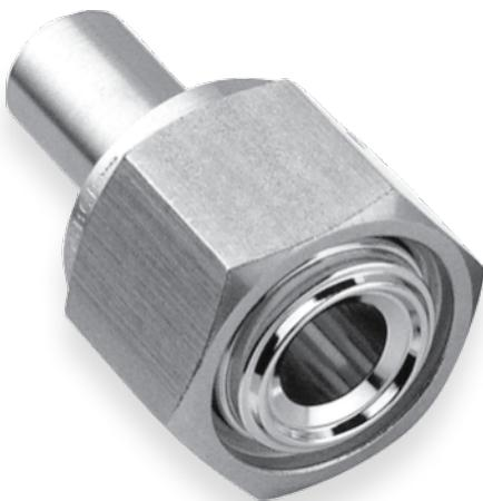
GENTEC® specializes in designing and manufacturing high quality valves and fittings for High Purity and Ultra-High Purity applications. GENTEC® FSR fittings are available in 316, 316L, or 316 VAR and supplied in BA or EP grade. Fittings are cleaned, bagged individually in nylon bags, and heat-sealed. The inner bag is then placed in a polyethylene outer bag and heat-sealed in a class 100 clean room to meet this stringent demands of the semi-conductor industry.
