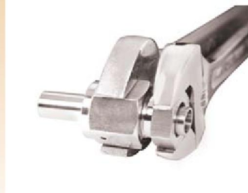
Holding the backup wrench stationary, tighten the female nut 1/8 turn past fingertight.
